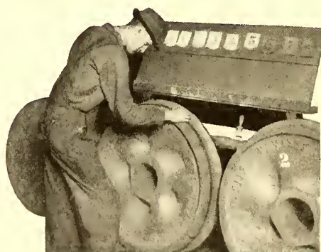
Taping Davis Steel Wheels to insure proper mating in service
